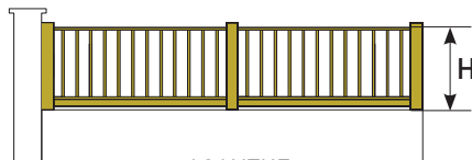
ACANTHE with grooved bars Ø 23,5 mm Space between bars 102 mm
