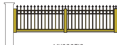
MYOSOTIS with grooved bars Ø 23,5 mm Space between bars 102 mm
